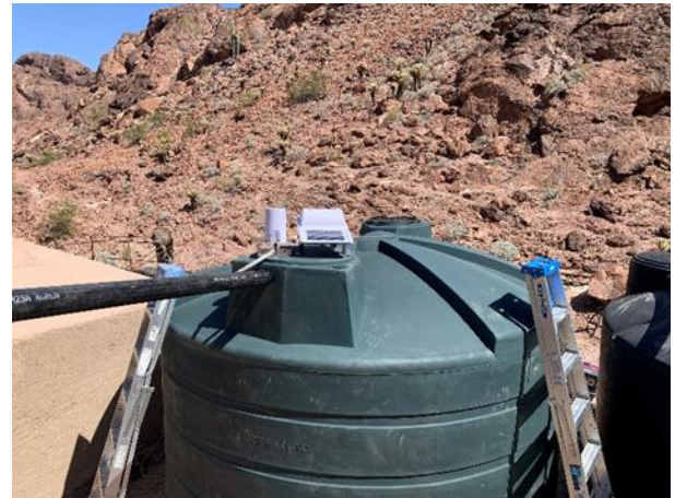
FIGURE 6. An example of a remote sensing device at a desert bighorn sheep water source. Once installed, this system communicates via satellite with a monitoring computer, and data such as water level and system failures can be detected without costly and time-consuming field visits.
